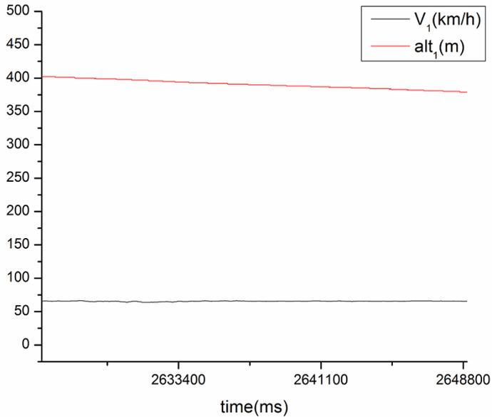
Fig. 4 Airspeed and altitude drop for the second gliding segment
