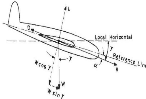
Fig. 2 Forces and angles for gliding flight
