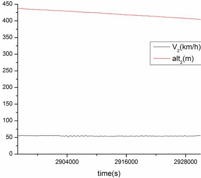
Fig. 5 Airspeed and altitude drop for the third gliding segment
