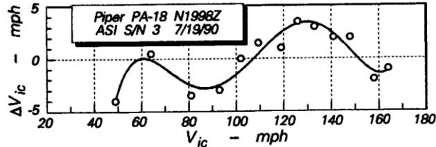
Fig. 1 Typical altimeter correction
