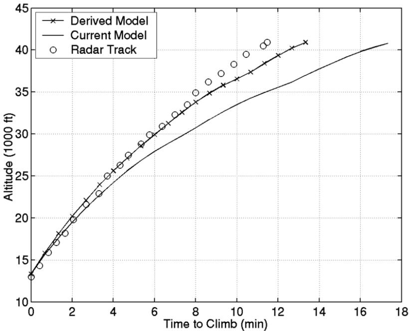
Fig. 9 Radar track vs aeropropulsiv model [1]
