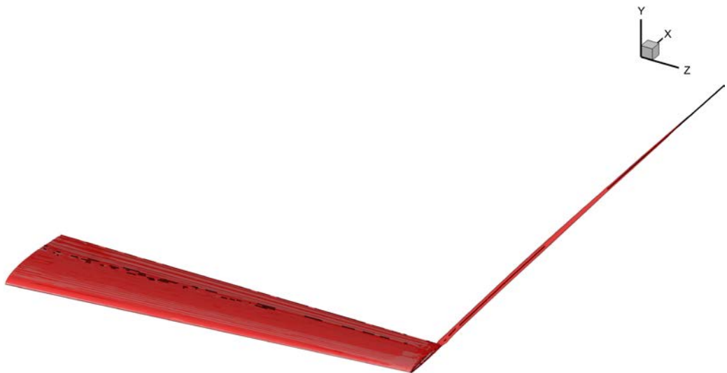
Fig. 12 Flow visualization of the wing tip vortex at \alpha = 0^\circ and Re = 1.0 \times 10^6
