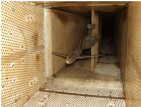
Fig. 2 ONERA M4R wind tunnel model in the transonic experimental chamber
