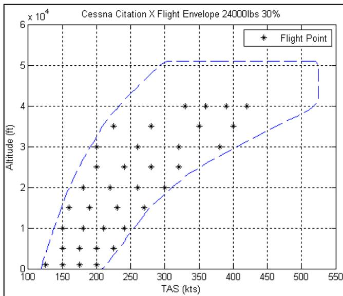
Figure 3. Cessna Citation X Aircraft Flight Envelope
