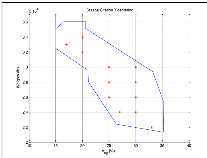
Figure 4. Cessna Citation X Weight/Xcg conditions
