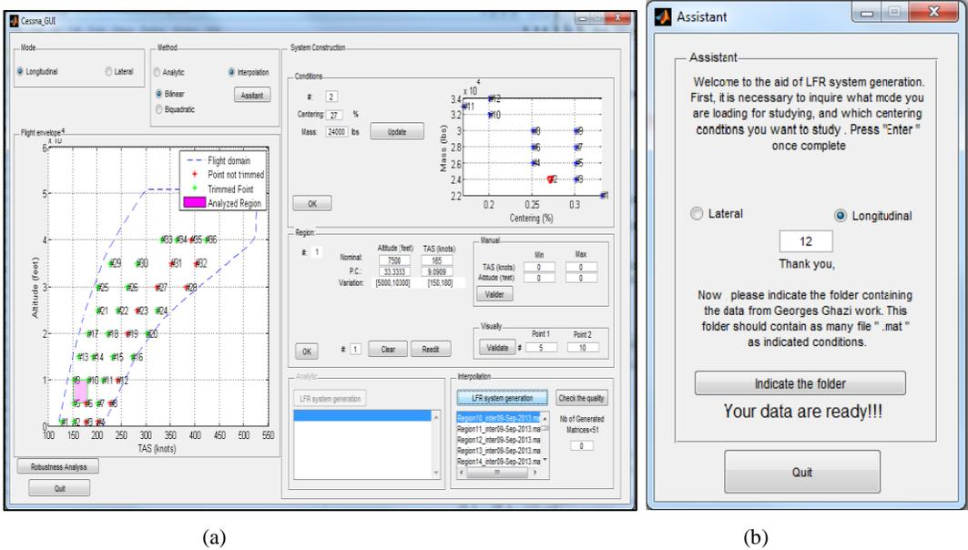
Figure 7. Graphical User Interface for generating the Cessna Citation X LFRs.
