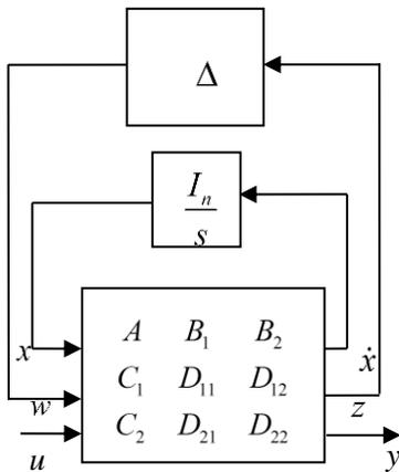
Figure 1. LFR of  $K(\frac{1}{s}, \delta_1, \dots, \delta_q)$  transfer function
