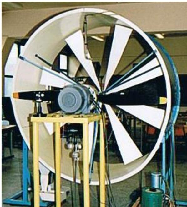
Fig. 7 The experimental stand for the propeller with 2m and 8 blades
