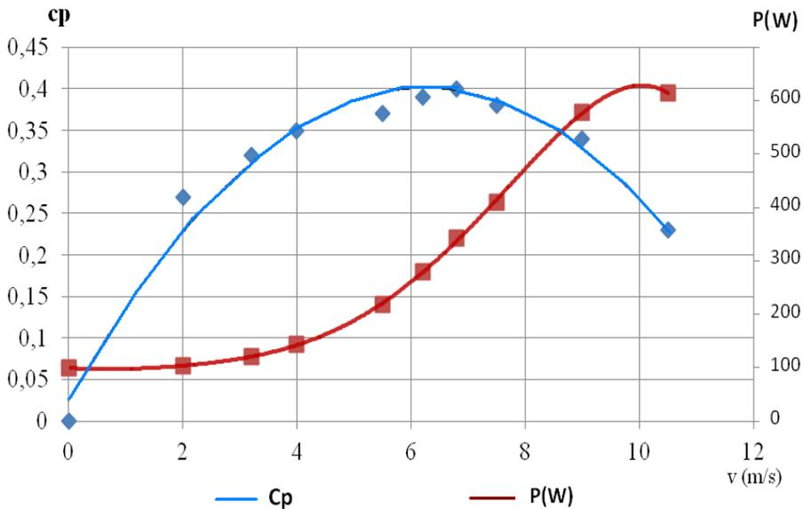
Fig. 6 Power curve and power coefficient relative to the wind velocities for the impeller with 8 blades and diameter of 2m
