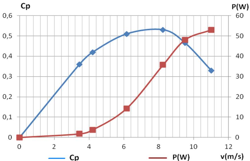
Fig. 5 Aerodynamic tests of the propeller with 4 blades and 0,5 m diameter - Variation of the  $c_p$  and  $P(W)$  with the air flow velocity
