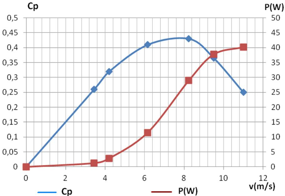
Fig. 2 Aerodynamic tests of the propeller with 3 blades and 0,5 m diameter - Variation of the  $c_p$  and  $P(W)$  with the air flow velocities
