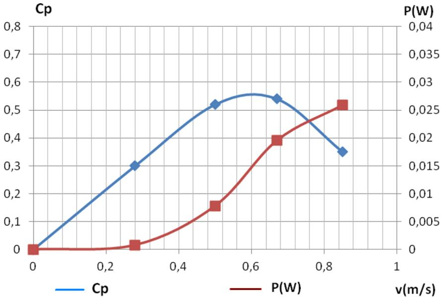
Fig. 4 Hydrodynamic tests of the impeller with 4 blades and 0,5 m diameter - Variation of the  $c_p$  and  $P(W)$  with the water current velocity
