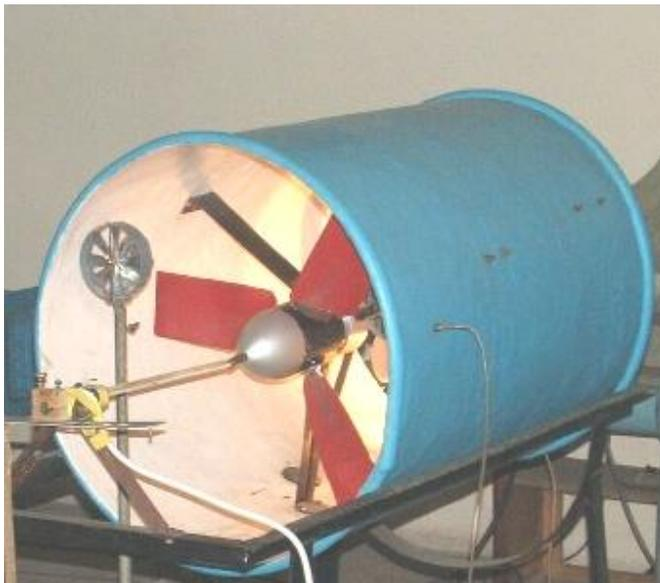
Fig. 3 The experimental stand with wind tunnel and the propeller with 3 blades
