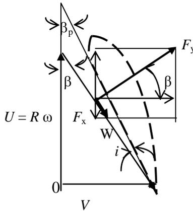
Fig. 1 Velocity triangle and the components of aerodynamic resultant
