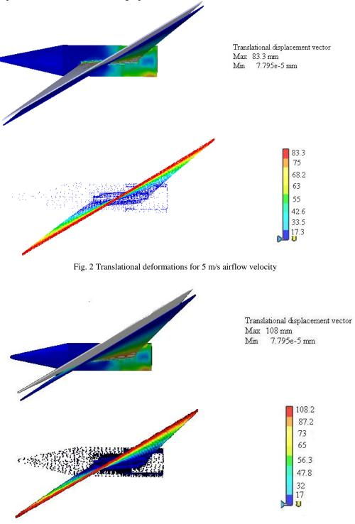
Fig. 3 Translational deformations for 10 m/s airflow velocity
