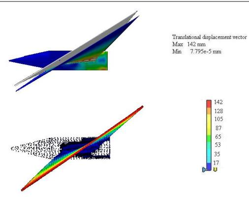
Fig. 4 Translational deformations for 20 m/s airflow velocity
