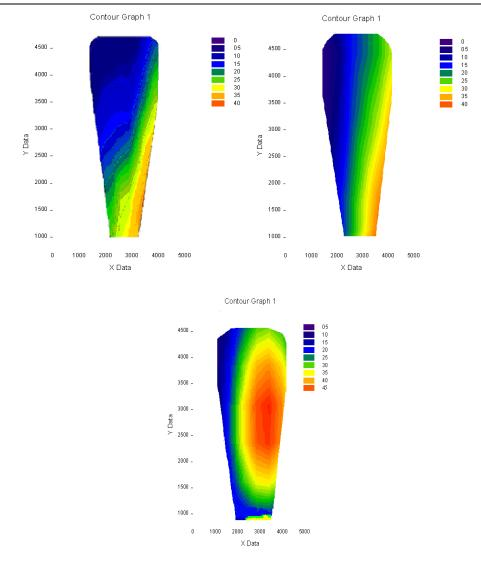
Fig. 1 Velocities spectrum in axial relative motion, for wind speeds of 0,5 m/s, 1 m/s , 3 m /s, 4 m/s and 5 m/s
