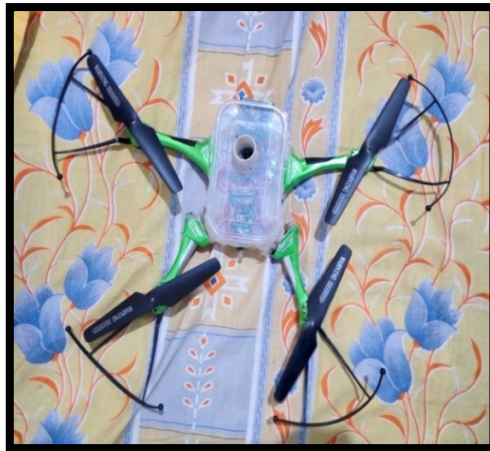
Figure (b): Unmanned Aero-amphibious Vehicle
