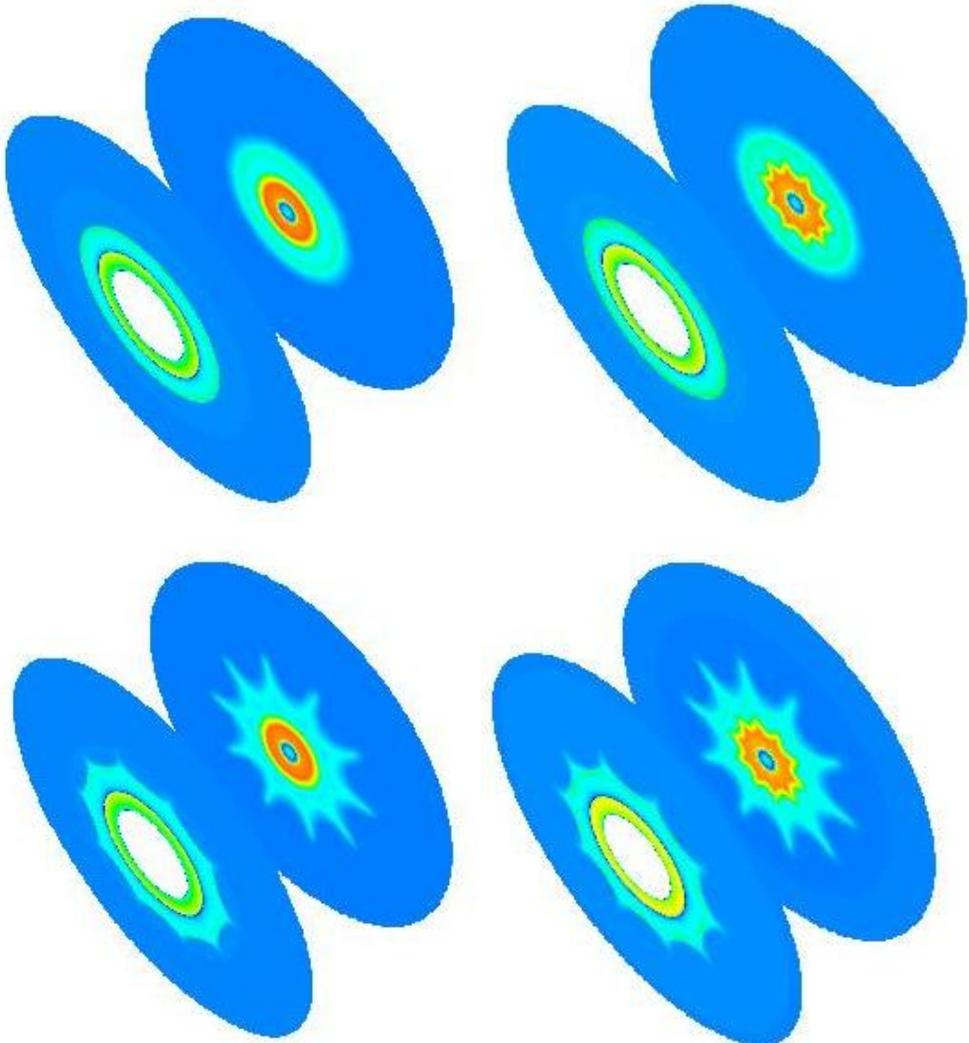
Fig. 9 Velocity distribution for ten chevrons for two different sections of the computational domain at 0.2 and 1.5 meters
