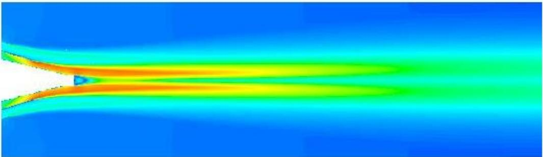
Fig. 7 Velocity distribution along the Ox axis for the nozzle
