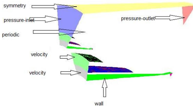
Fig. 6 The boundary conditions for the computational domain
