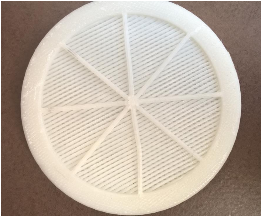
Fig. 8 – Final part with fine layers extracted from the base plate
