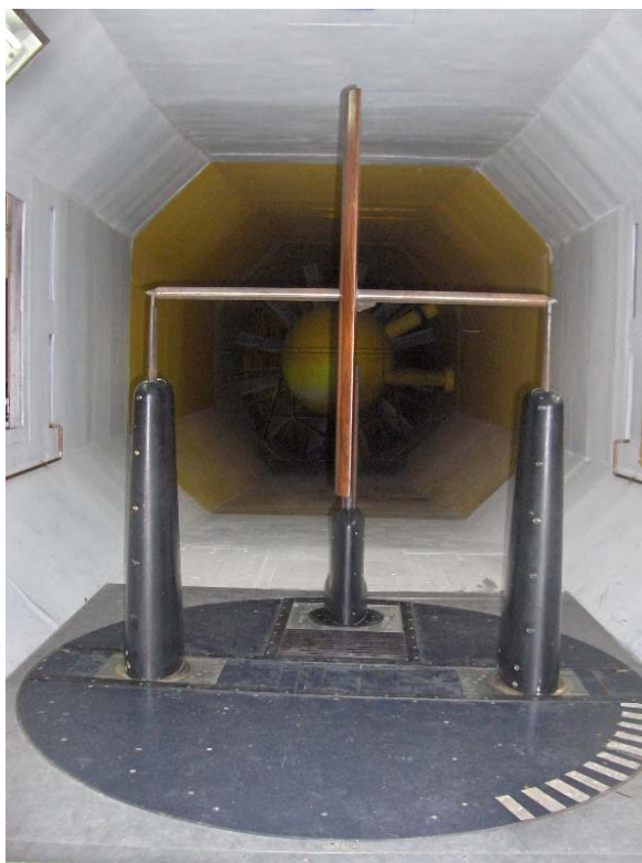
Fig. 4 – Experimental assembly for determination of horizontal deflection
