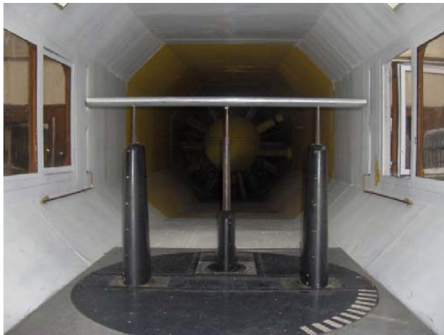
Fig. 3 – Experimental assembly for determination of vertical deflection
