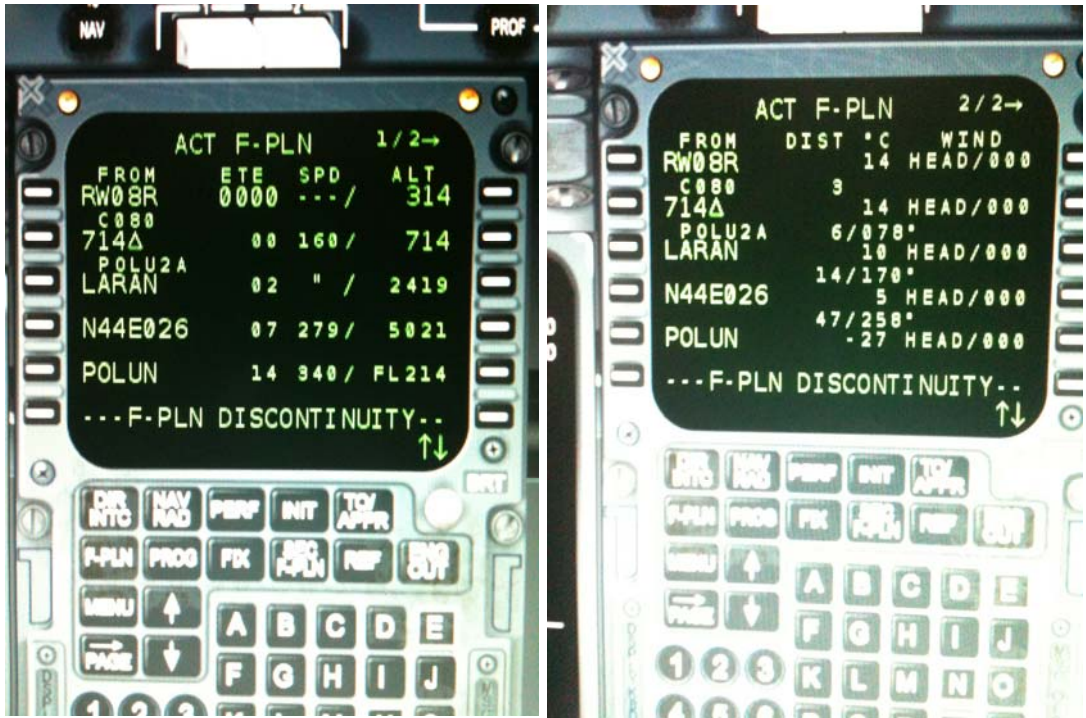
Configuration of the FMS for the actual standard instrument departure route POLUN2A
