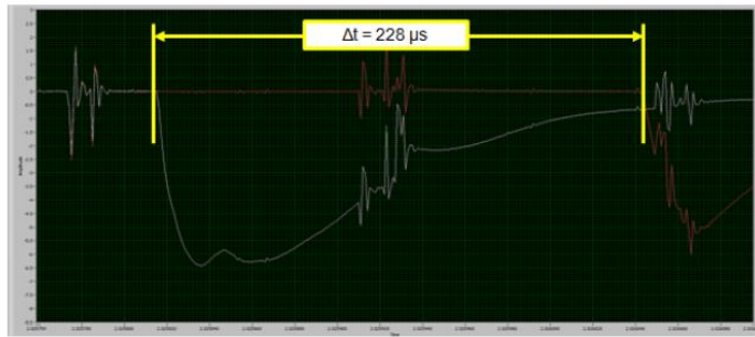
Figure 4. Wave traces after DDT from a pair of ports separated by four inches [31]
