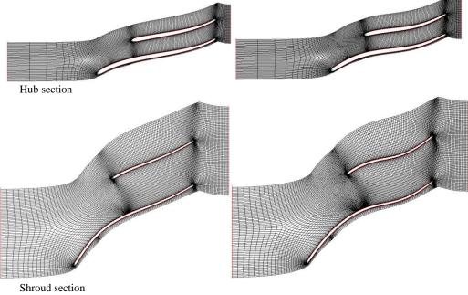
Fig. 5 - b. The optimal rotor geometry compared with the initial rotor
