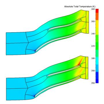
Fig. 8 - Absolute total temperature flow field of the optimized (top) and baseline (bottom) rotor in the midspan section (blade to blade view)
