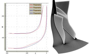
Fig. 5 - a. The optimal rotor geometry compared with the initial rotor
