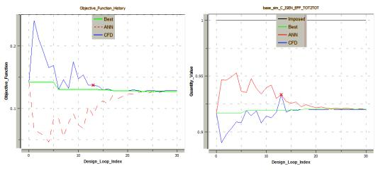
Fig. 3 - Objective function and isentropic efficiency vs. optimization attempt index
