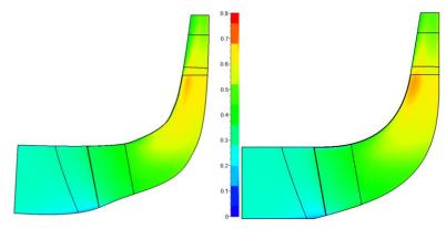
Fig. 6 - Absolute Mach number across the channel Optimized (left) and baseline (right) meridian plane
