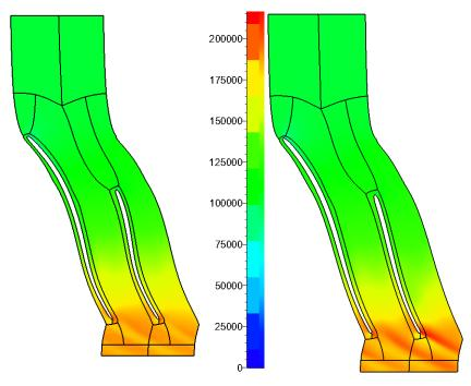
Fig. 7 - Absolute total pressure blade to blade Optimized (left) and baseline (right) midspan section
