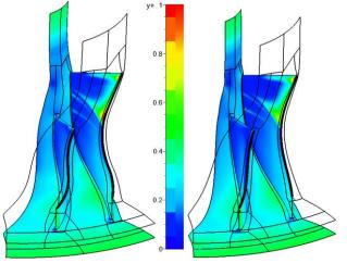
Fig.4 - The y+ distribution near the walls of the rotor Optimized (left) and baseline (right)
