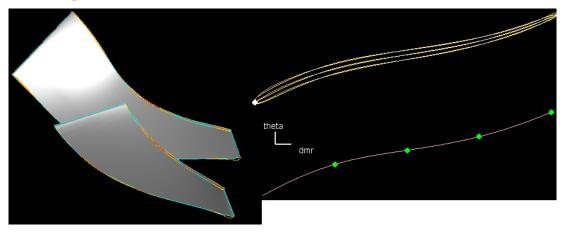
Fig. 2 - The fitted geometry overimposed on the baseline geometry
