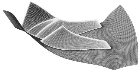
Fig.1 - Solid mesh near the walls of the rotor for a channel
