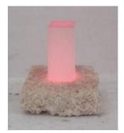
Fig. 7 The sample after the first test (25 h in furnace)
