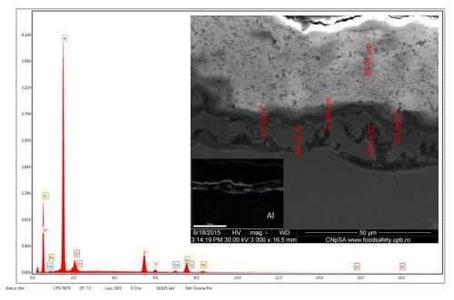
Fig. 12 Specimen microstructure after 250 h of testing (10 cycles)
