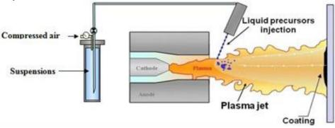
Fig. 2 Suspension plasma spray deposition [6]
