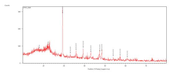
Fig. 13 X-Ray Diffraction of thermal barrier coating MeCrAlY / ZrO28% Y2O3 of sample after 250 h testing (10 cycles) at 1000°C
