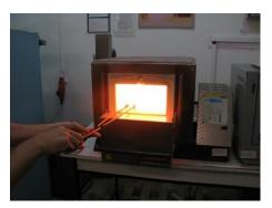
Fig. 6 Removing the sample from the furnace
