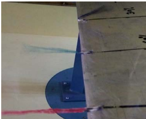
Figure 4. Flat plate tuft at 6^\circ AOA, Re_c 2.25 \times 10^5
