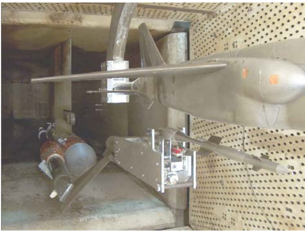
Fig. 4 . Captive Trajectory Simulation system
