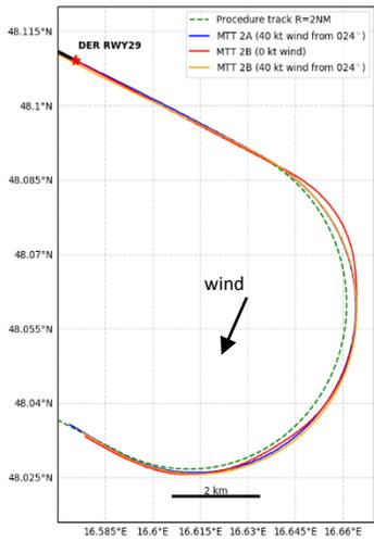
Fig. 7 – Flight tracks for the SIDs with 2 NM turn radius under wind and still-air conditions
