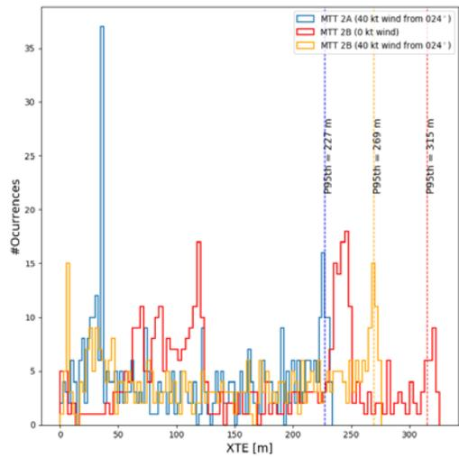
Fig. 8 – XTE histograms (P95) for the SIDs with 2 NM turn radius in still air and with wind
