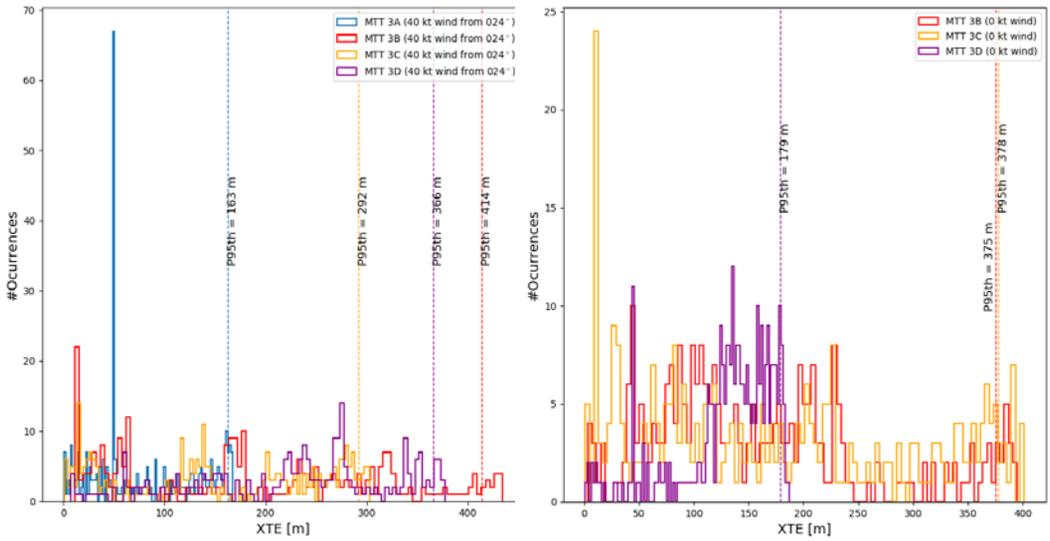
Fig. 5 – XTE histograms (P95) for the SIDs with 3 NM turn radius in still air (right) and with wind (left)
