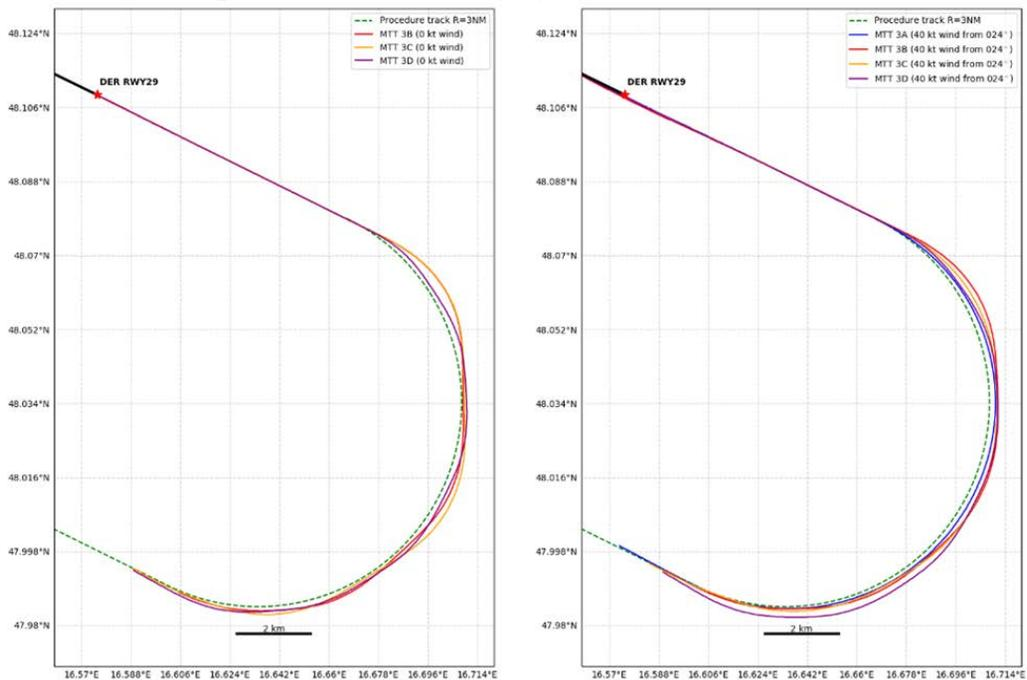
Fig. 4 – Flight tracks for the SIDs with 3 NM turn radius under wind and still-air conditions
