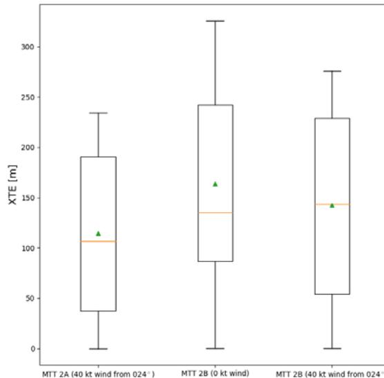
Fig. 9 – Box-and-whiskers plot showing range, quartiles and mean for the distribution of XTE values during the test flights of the SIDs with 2 NM turn radius under wind and still-air conditions
