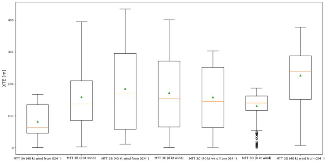
Fig. 6 – Box-and-whiskers plot showing range, quartiles and mean for the distribution of XTE values during the test flights of the SIDs with 3 NM turn radius under wind and still-air conditions
