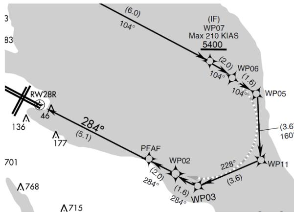
Fig. 1 – Established-on-RNP overlay approach based on TF legs [17]
