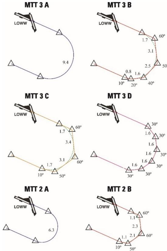
Fig. 2 – MTT sequences with the corresponding track changes (segment lengths are shown in NM)
