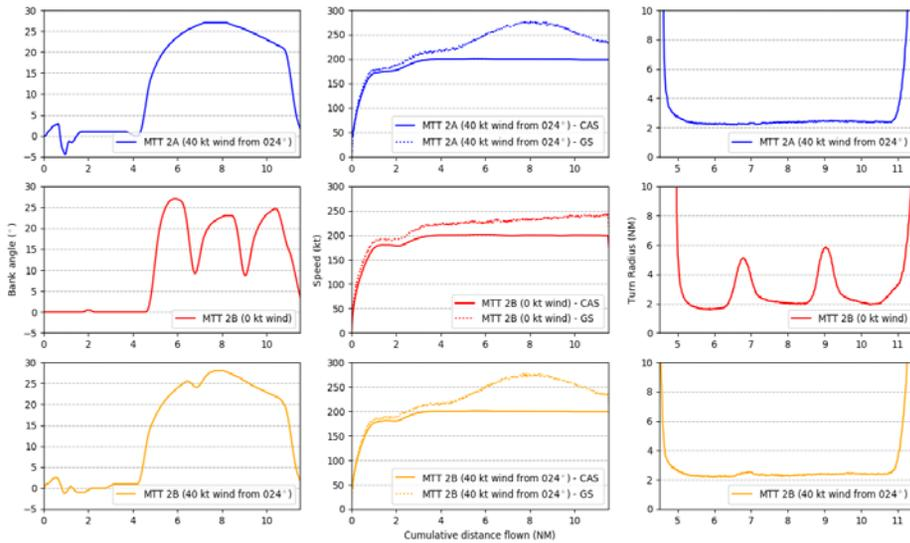
Fig. 10 – Actual turn radius, speed and bank angle for the SIDs under wind and still-air conditions
