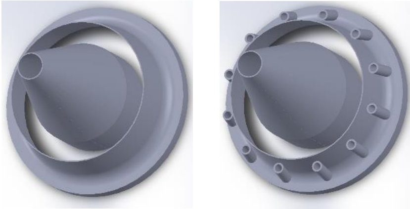
Figure 7. The CAD models of the 2 configurations: base model and 12 chevrons
