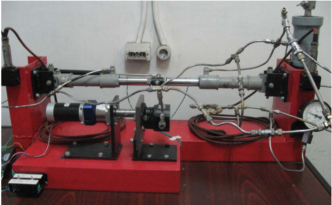
Fig. 7. View of the test rig for the hydrostatic actuator
