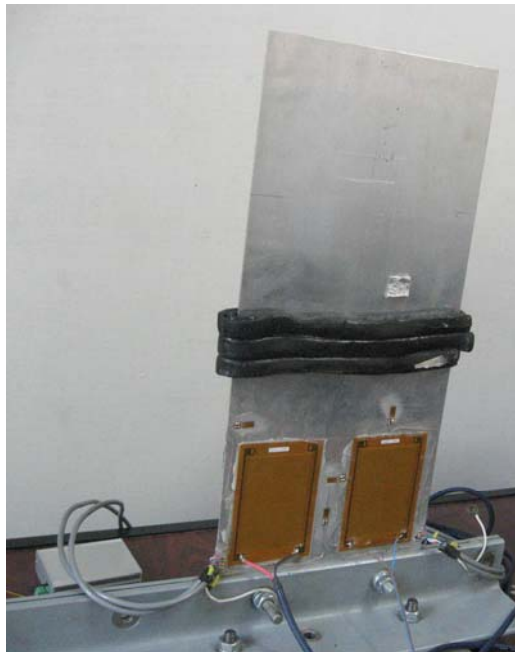
Fig. 1 – Photo of the assembly duraluminum cantilever plate with MFC and lute bandage for simulation of modal type damages
