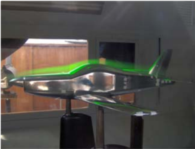
Fig. 5 - Visualization of air flow performed with longitudinally oriented laser light sheet. The air flow lines with seeding smoke near the aircraft model surface are indicated with an arrow. The attack angle of the aircraft model versus the airflow direction is \sim 2^\circ . The air flow speed is 15 m/s.
