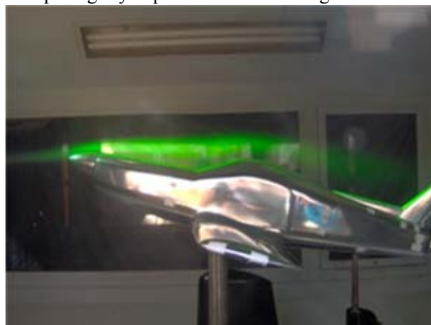
Fig. 4 - Visualization of air flow performed with longitudinally oriented laser light sheet. The air flow lines with seeding smoke near the aircraft model surface are indicated with an arrow. The attack angle of the aircraft model versus the airflow is of \sim 35^\circ . The air flow speed is 15 m/s.
