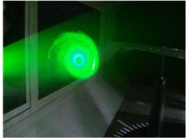
Fig. 7 - Visualization of air flow performed with transversally oriented laser light sheet. The air flow lines with seeding smoke are indicated with an arrow. The air flow vortex appearing at the end of aircraft model wing is indicated with an arrow. The attack angle of the aircraft model versus the airflow is of \sim 35^\circ . The air flow speed is 15 m/s.
