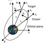
Fig. 2 Chaser and target vehicles orbit. Reference system centred on the target vehicle
