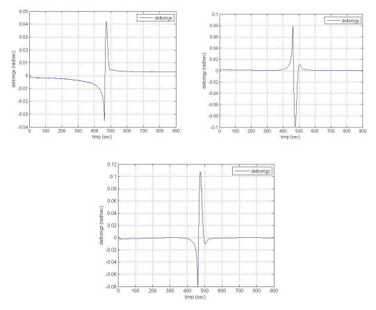
Fig. 7 SDRE control attitude rates error
