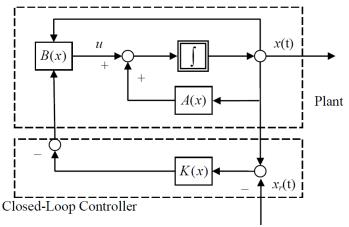
Fig. 4 Block diagram of the SDRE Control
