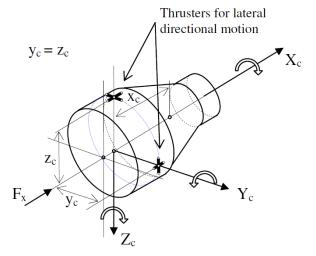
Fig. 3 Generic model proposed for attitude dynamics with controls
