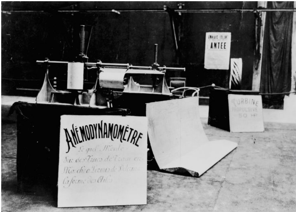
Measuring apparatus – Anemo-dynamometer
