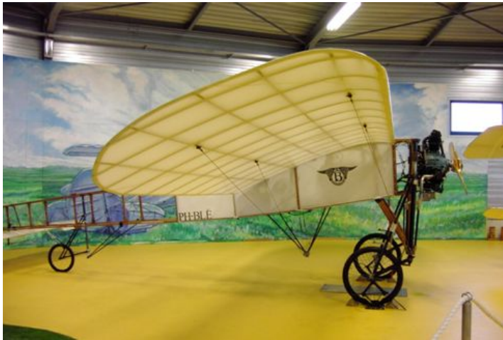
Bleriot XI monoplane. Note the wing profile.
