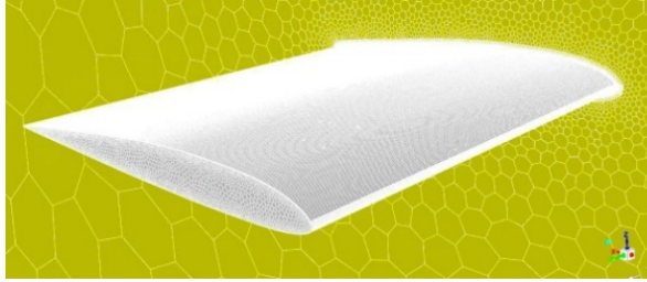
Fig. 6 Mesh grid model of the UAS-S45 wing
