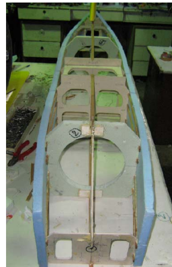
Fig. 2 Fuselage in the early stage
