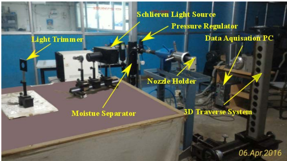
Fig. 1 Experimental Setup (supersonic Jet Facility at Madras Institute of Technology)
