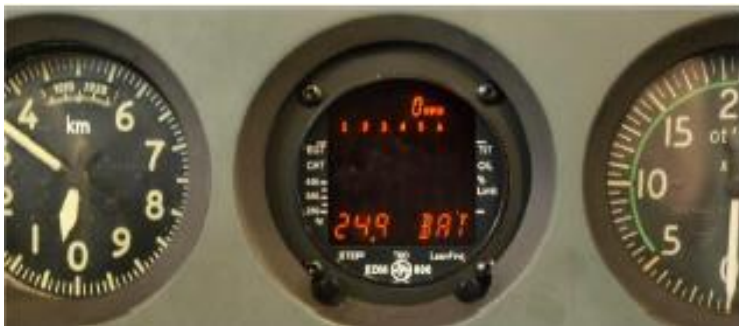
Figure 3. EDM-800’s emplacement on the instrument panel in Zlin 43 (Kříž et al, 2010)
