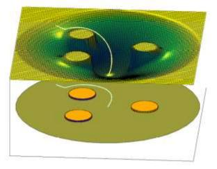
Fig. 6 - Navigation Function with three obstacles and the resulting gradient following path
