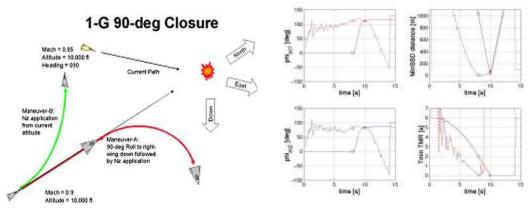
Fig. 9 - ACAS scenario simulation in D-SIX environment
