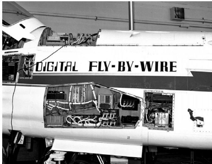
Fig. 4 F-16 fighting falcon fly-by-wire system [4]
