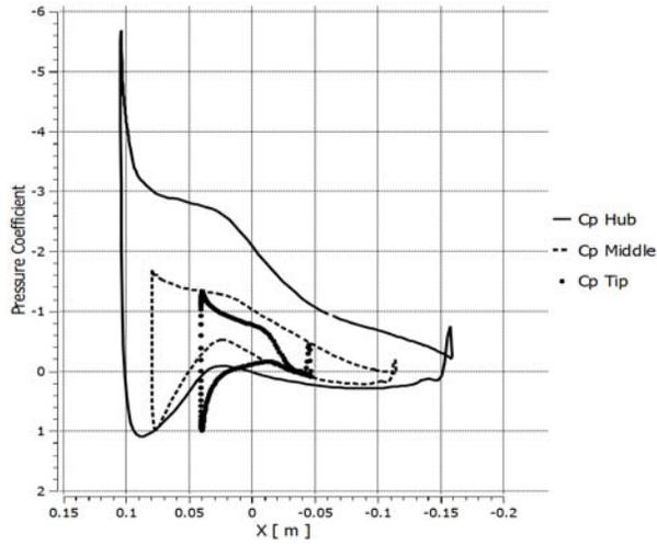
Fig. 1 – Pressure coefficient with respect to relative velocity, near hub, midspan and tip, at wind velocity of 8 m/s and tip speed ratio of 6, computed with in-house code, using RANS approach
