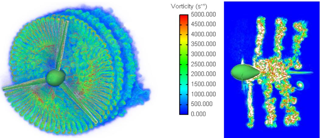
Fig. 3 – The evolution of vorticity after 1 revolution of wind turbine rotor, at wind velocity of 14 m/s and tip speed ratio of 6, computed with XFlow, using LES approach
