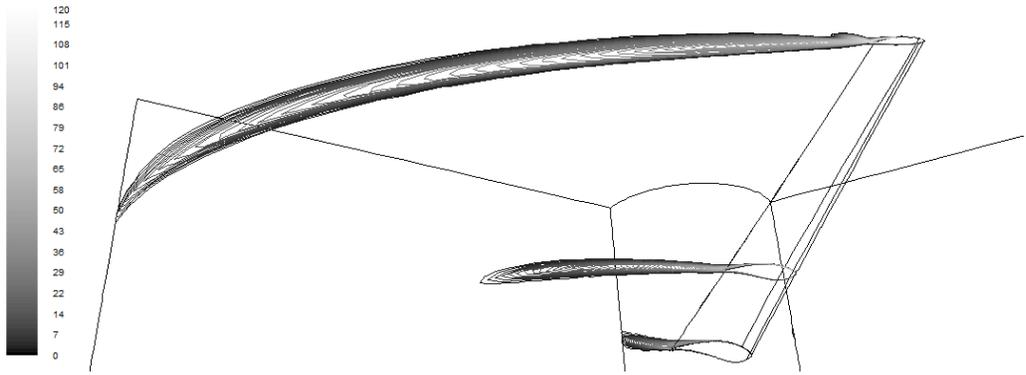
Fig. 2 – Isolines of acoustic power level (dB) near hub, midspan and tip, at wind velocity of 8 m/s and tip speed ratio of 6, computed with in-house code, using RANS approach
