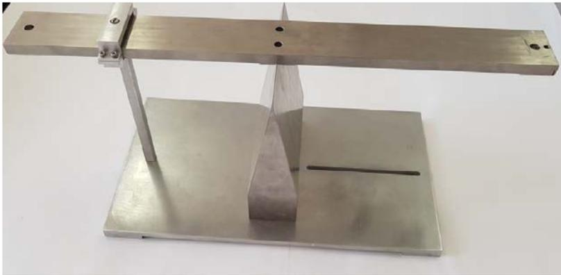
Fig. 7 – Realized and assembled balance components
