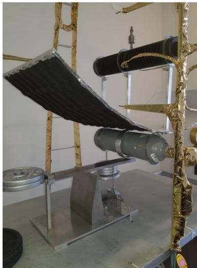
Fig. 8 – Satellite propulsion fixed on balance [5]
