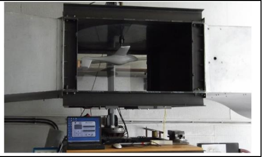
Fig. 4 - The model within the wind tunnel test section
