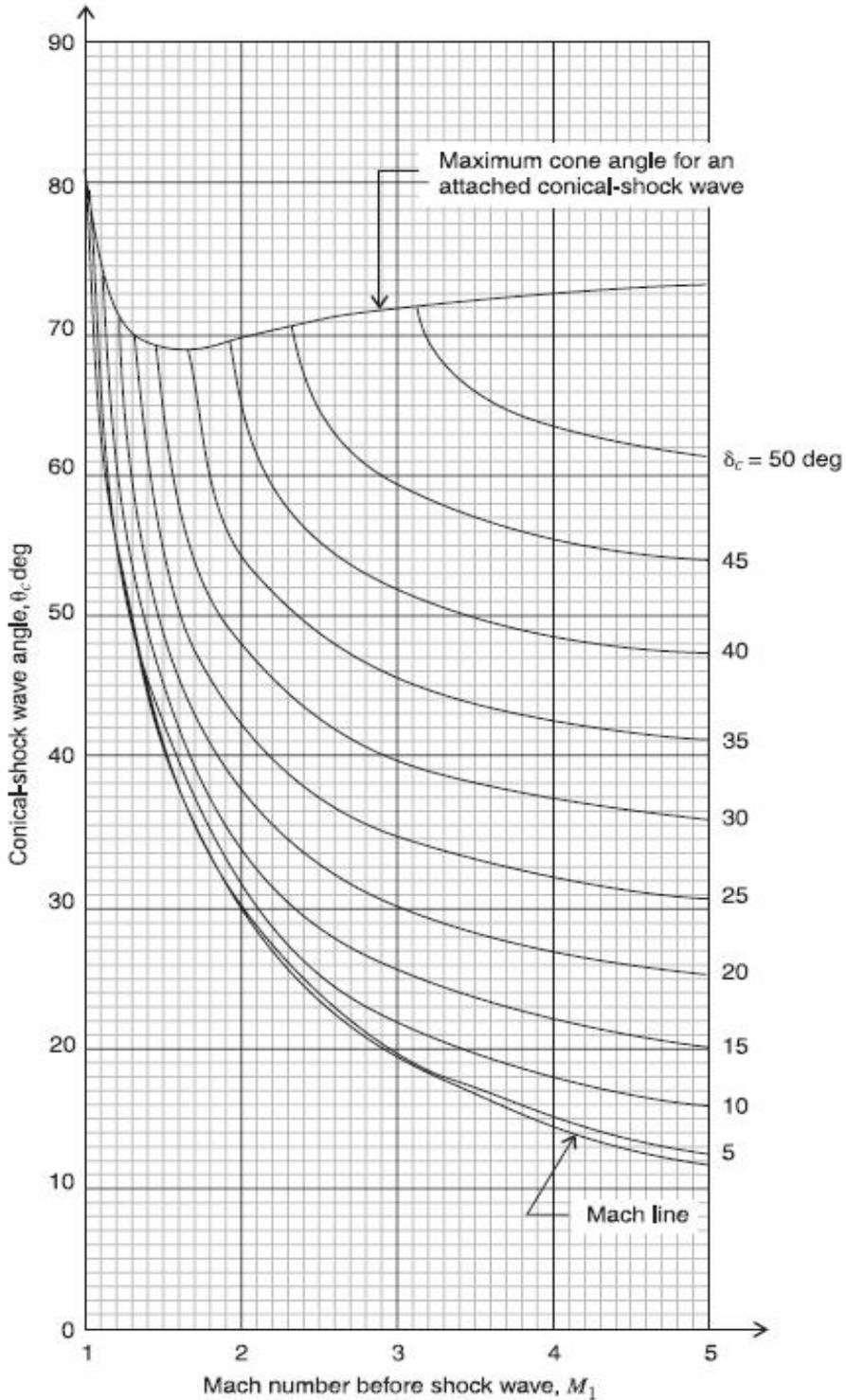
Figure 4. Finding the Mach number by Schlieren photogrammetry is made possible by charts like these [5], [6] We solve the equation numerically to get  $V_r$  and an angle  $\theta$  for which  $V_\theta = 0$ , that would give the speeds behind the shock wave having that angle. The method is solving numerically for a
