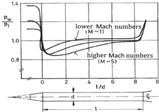
Figure 2. The theoretical pressure distribution for a cone-cylinder probe is taken as reference for the validation of the experimental conditions of the supersonic Pitot tube measurements [3]
