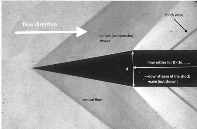
Figure 3. A cone-cylinder probe head in supersonic flow. Note the system of the simple waves and the thin shock wave that forms approximately at 2d from the cone-cylinder junction
