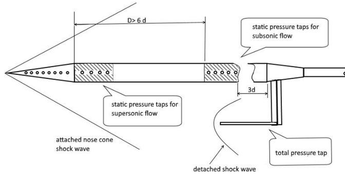
Figure 1. The modified cone-cylinder probe is transformed in a supersonic Pitot tube with expanded capabilities in transonic and subsonic regimes if appropriate selection of static pressure taps is made
