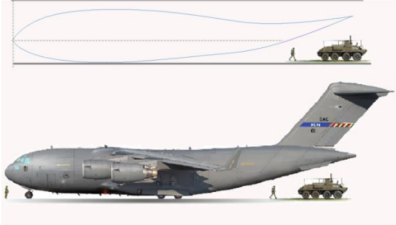
Fig. 8 – Comparison of C17 fuselage shape with scaled reflex airfoil
