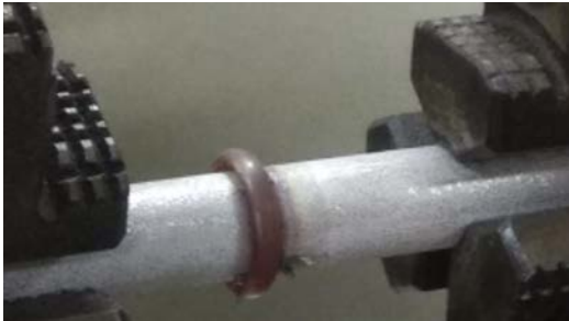
Fig. 5 Welded dissimilar materials of titanium and stainless steel with an aluminium coating
