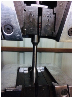
Fig. 7 Tensile test setup of UTM
