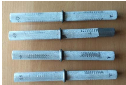
Fig. 6 Heat treatment welded samples of Ti-6Al-4V and SS304L
