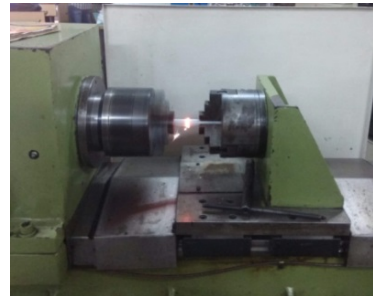
Fig. 4 Initial Fire point of the frictional welding process
