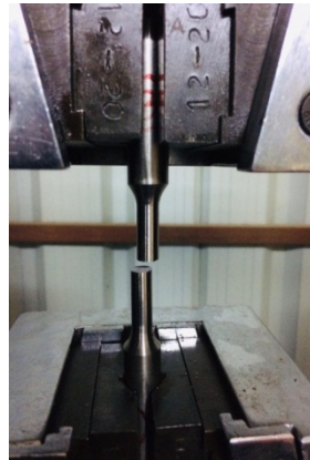
Fig. 8 Tensile broken area view
