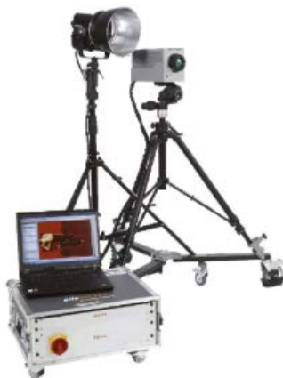
Fig. 14 Installation used for active thermography [21]
