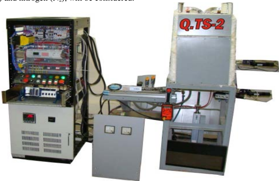
Figure 2. - QTS-2 Rapid Heat Shock equipment
