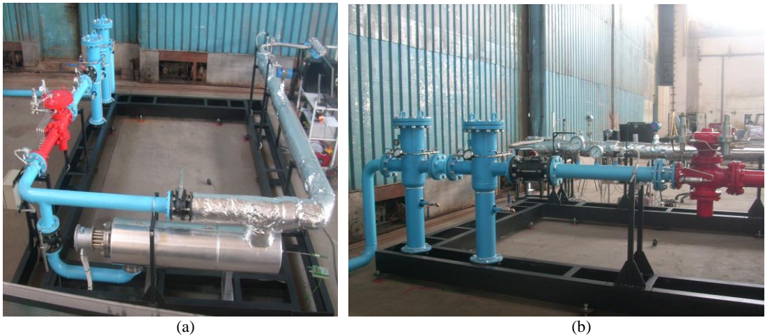
Figure 3. General view of the system (a) and air filtering units and pressure regulator (b)
