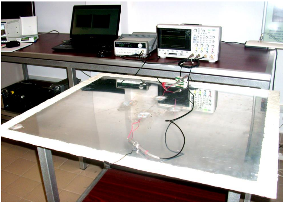
Fig. 5 The experimental system setup for tuning Lamb waves
