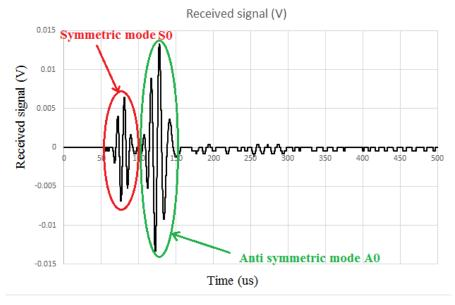
Figure 7. Antisymmetric A0 and symmetric S0 modes [7]
