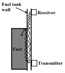
Figure 2. Propagating waves through the system
