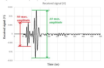
Figure 8. Measuring A0 and symmetric S0 modes signal maximum amplitudes
