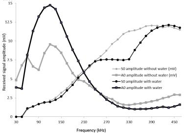
Figure 9. Dependence of the amplitude of the received signal with frequency
