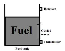
Figure 1. Schematics of the method setup
