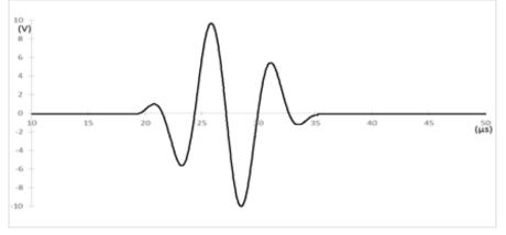
Figure 6. Hanning window modulation sinusoidal pulse [6]
