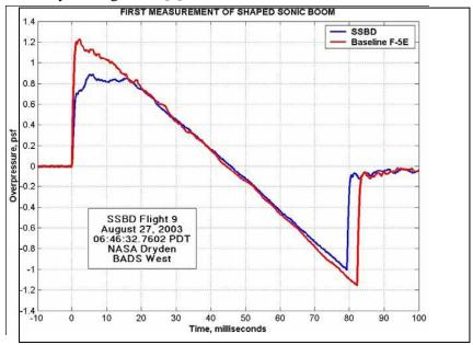
Figure 7: First measurement of shaped sonic boom of F-5E aircraft modified by Northrop Grumman (blue: shock wave after shaping)
