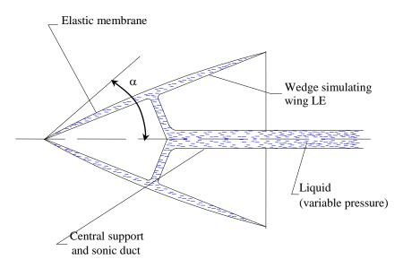
Figure 11: Variation of  $\alpha$  at the preliminary design solution
