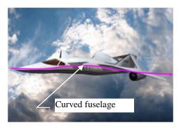
Figure 6: Curved fuselage – Lockheed Martin early concept
