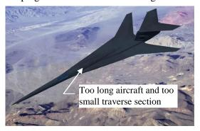
Figure 5: Thin and long aircraft – Lockheed Martin early concept
