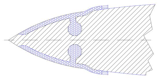
Figure 13: Scattering of shock wave by means of vibration of elastic plates induced by compressed air
