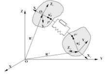
Fig. 2 Linear spring and damper connection
