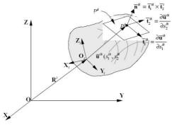
Fig. 6 Contact connection
