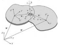
Fig. 5 Revolute joint connection
