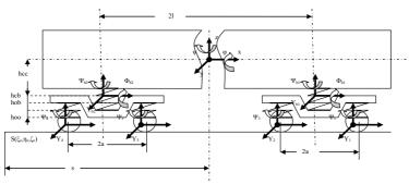
Fig. 7 Mechanical model for passenger coach's hunting (lateral view)
