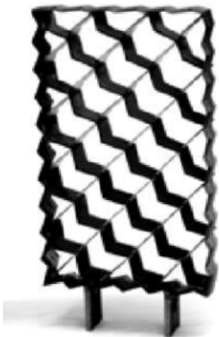
Figure 3: A locally sweptback grid fin model configuration [19]
