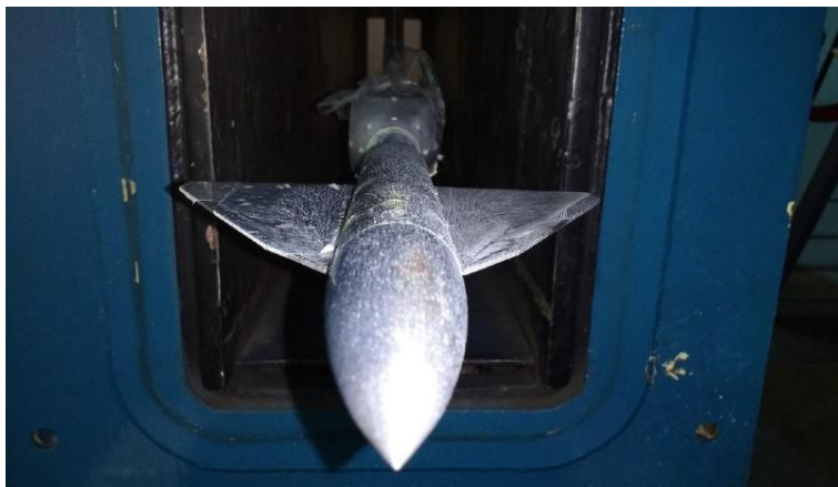
Figure 1 - Entire Model of the Compound Delta Wing with setup
