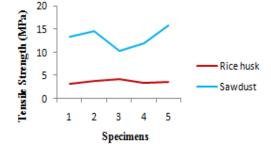
Fig. 7 Comparison of Tensile strength of different fiber sheets for different samples
