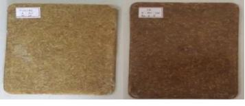
a) Resin: Rice Husk b) Resin: Saw Dust 90:10 90:10 Fig. 6 Photograph of laminates: a) PR+RH and b) PR+SD
