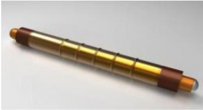
Fig. 8 - Geiger tube designed in CAD
