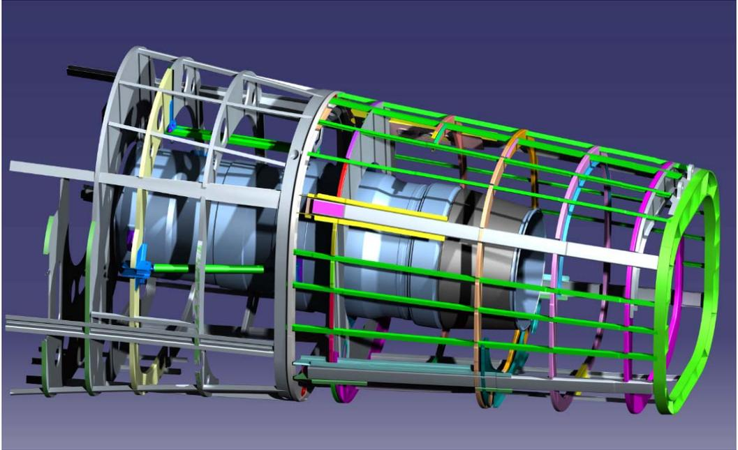
Engine Installation in Fuselage
