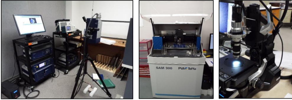
Fig. 4 – LAMSS, UofSC equipment used in the project; left: Scanning Laser Doppler Vibrometer (SLDV; Polytec PSV-400); middle: SAM 300 scanning acoustic microscope ( http://www.pva-analyticalsystems.com ); right: digital microscope VHX 5000 ( www.keyence.co.uk/ )
