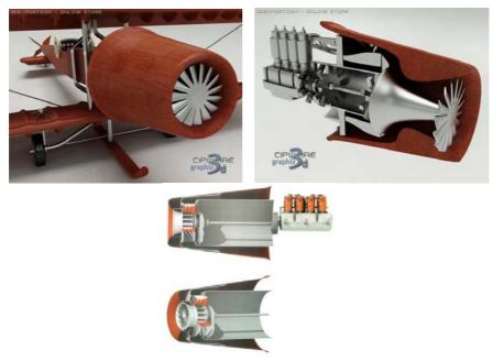
Fig. 8-3D Model of Coanda's engine
