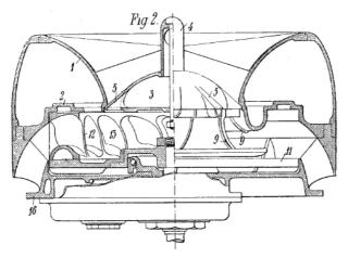
Fig. 5- Centrifugal compressor (two known variants)
