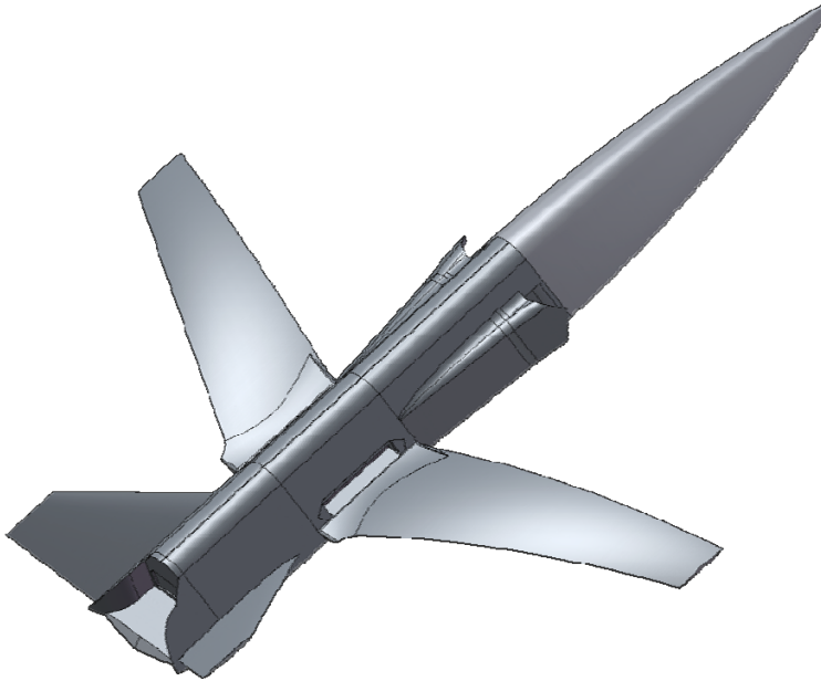
Fig.1 Axonometric view of the stealth hovering UAV concept
